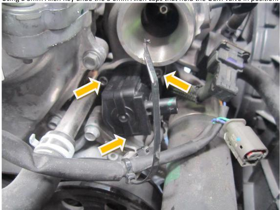
7. Once the OEM valve is removed place the Forge Motorsport valve into position ensuring the O-rings are in place and tighten the allen cap bolts.
