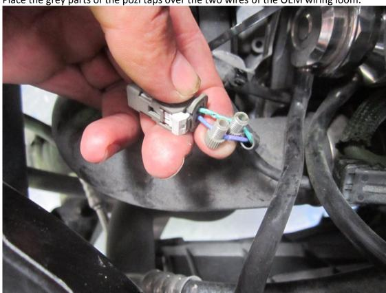
11. Screw the middle part of the pozi tap into the grey connectors with the point end in first.
