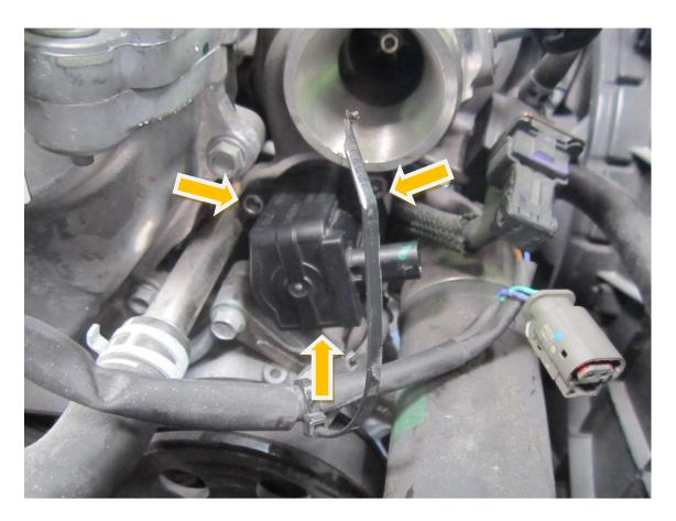
7. Ensure the O-rings are in place and fit the Forge Motorsport valve into position using the three OEM bolts.
