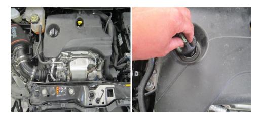
2. Remove the engine cover by pulling upwards sharply.
