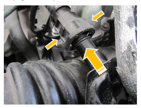
5. Once the inlet hose is removed you will be able to gain access to the OEM dump valve, unclip the wiring connector from the OEM dump valve by pushing on the tab and pulling away.
