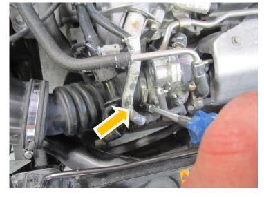
4. Undo the breather hose that feeds to the inlet hose, press on the tabs either side of the mounting clip while pulling the inlet hose away.
