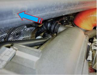
3. Unclip the vacuum hoses and wiring harness from the side of the boost pipe.
