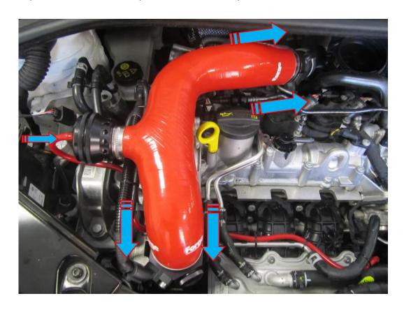
Fit the breather hose to the machined adaptor if your vehicle is so equipped.
