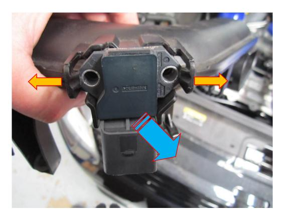
8. Fit the map sensor to the Forge Motorsport billet coupler as shown in the picture below. Use the two M6x12 Allen cap head fasteners provided to secure the map sensor, the blanking plug simply screws into the coupler in a clockwise direction.
