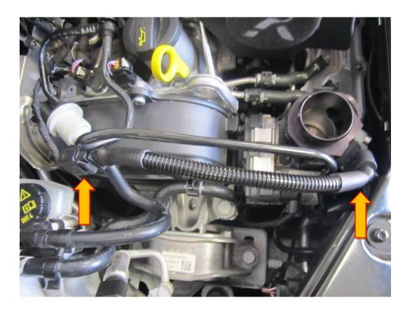
11. As pictured below remove the  $2^{\rm nd}$  map sensor from the inlet manifold.
