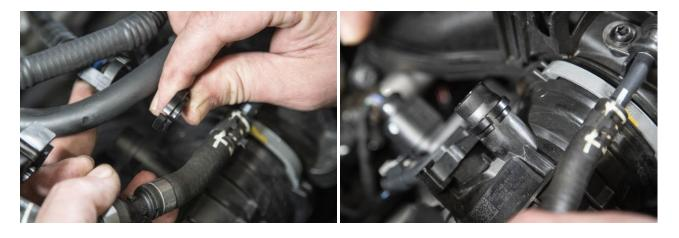
4. Push the supplied adapter over the pipe ensuring the slot is over the split sleeve.
