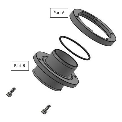
14. Align cut outs of Part A and place over the turbo outlet, turn approx 90 degrees. Then install Part B and bolt to Part A using the two M4 cap head fasteners supplied.
