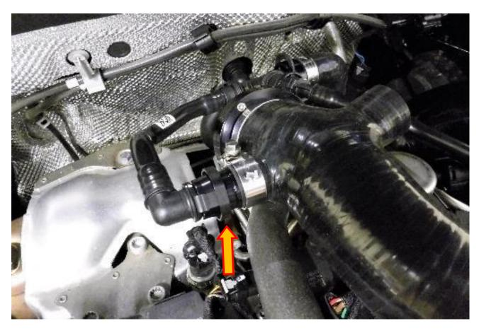
**18**. Fit the Forge Motorsport Valve from the FMDV39 kit then using the supplied 20-32mm hose clamp fasten in position.
