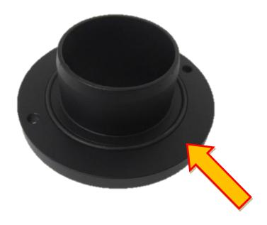
13. Attach the two pieces of the smaller Forge Motorsport billet coupler together using the two M4 fasteners supplied, use a 4mm Allen key to tighten, however only loosely fit them at this stage.
