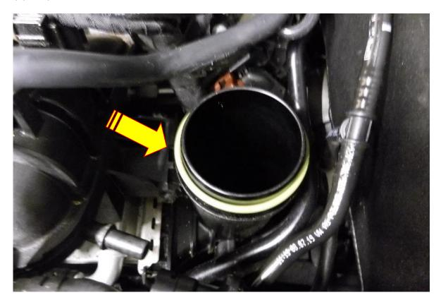
**11**. Fit the larger single piece Forge Motorsport billet coupler over the charge cooler inlet pipe and secure in place with the OE plastic retaining clip.
