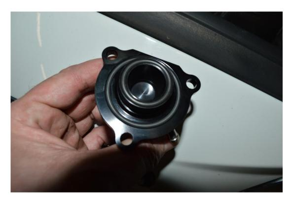
7. Using the original fasteners fit the Forge valve to the turbo.
