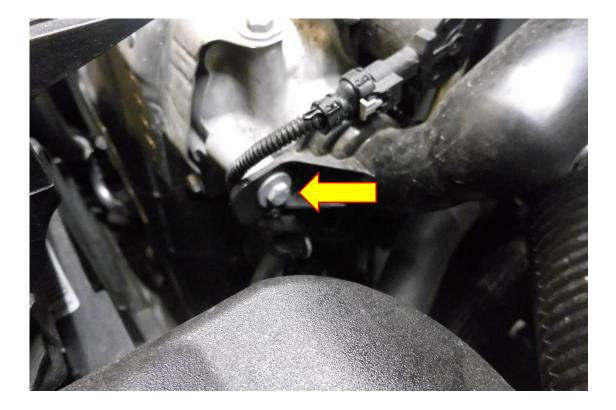
3. Press in both small tabs to remove the small breather and pull the yellow tabs apart to remove the large breather. You will now be able to pull the turbo inlet to the side.
