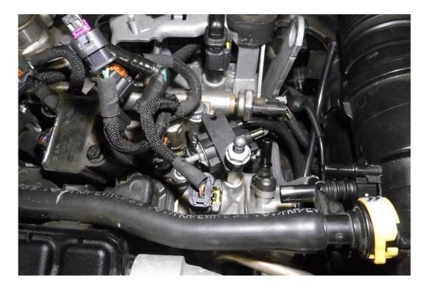
**11**. Route the vacuum hose to the boost solenoid provided and cut the tube to length attaching the vacuum hose to the solenoid as per the diagram pictured below.
