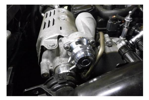
8. Press in the green locking tab at the end of the vehicles vacuum pipe and using a flat blade screwdriver release the retaining clip further down the pipe.
