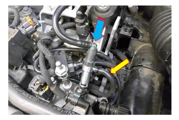
**16**. Using a T20 Torx drive remove the fastener attaching the air box lid. Take the supplied P clip and secure the vehicles vacuum line to the airbox lid and attach it using the same Torx fastener.
