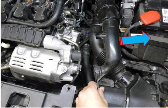
4. Pull the grey locking tab backwards and push the retaining clip in to remove the wiring loom attached to the OE valve.
