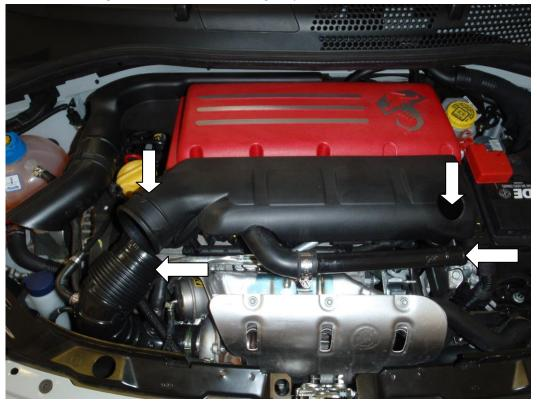
2. Using a T20 screw driver, remove the plastic bracket that retains the 3 hoses next to the oil dipstick, then using a T30 screw driver remove the MAP sensor from the inlet manifold.
