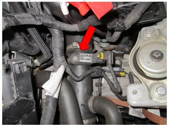
12. Place the Forge take off block **E** under the sensor and refit using screw A or C provided.
