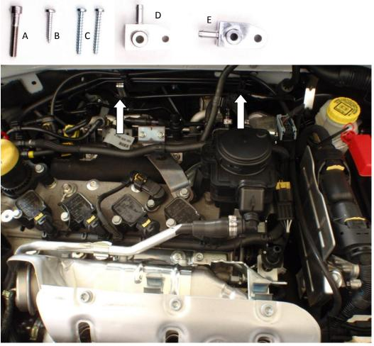
4. Connect the supplied length of silicon vacuum hose to the take off just fitted, and route it around the engine bay, using the clips already on the bulkhead to hold it in place, and route it between the ECU and the engine block to the front of the car by the stock valve. Use the supplied cable ties to secure it in the engine b
