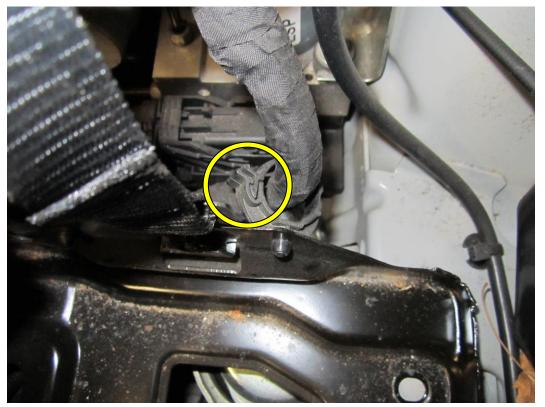
11. Now the battery tray has been completely removed locate the sensor that mounts on the boost pipe beneath. Using a T25 torx driver or Allen key, remove the sensor.
