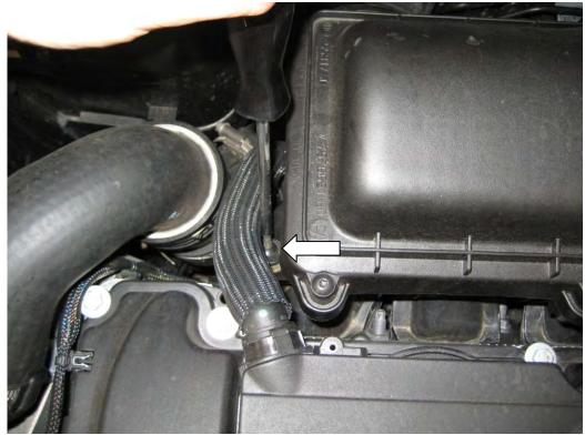
3. Remove the MAP sensor from the top of the inlet manifold as shown, then push it firmly into the supplied Forge MAP sensor boss. A little silicon spray will make it easier. Attach the length of silicon vacuum hose supplied to the vacuum nipple on the side of the boss, then reattach the whole assembly back to the inlet manifold with the brass screw provided.
