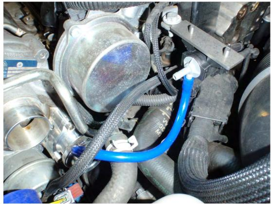
Cut a short length of vacuum hose and connect it between the dump valve TOP vacuum nipple and the vertical nipple on the solenoid. The dump valve nipple can be rotated around the body by loosening the top and rotating it. Connect the BOTTOM vacuum nipple on the dump valve to the METAL nipple on the solenoid.
