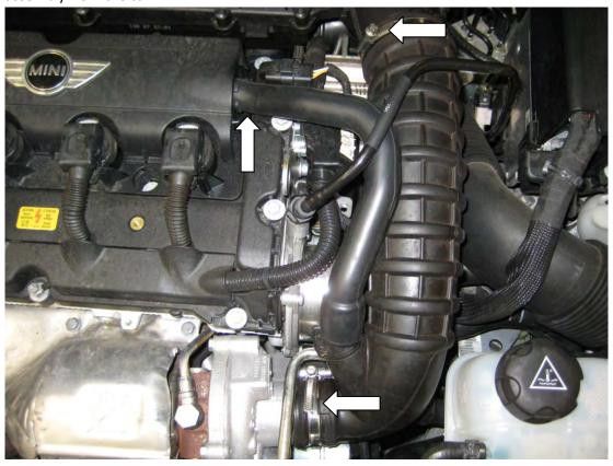
2. Remove the airbox by undoing the single bolt on the left hand side, then pulling it upwards to remove it from the rubber grommets that hold it to the top of the inlet manifold, giving you access to the cold air feed that simply pulls off the right hand side.
