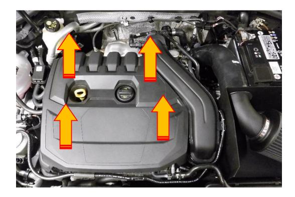
2. Remove the vacuum hose going into the inlet manifold by releasing the clip and pulling the hose away from the inlet, unclip the vacuum hose attached to the boost hose.
