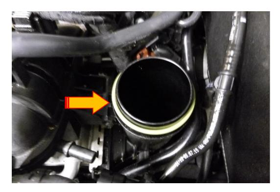
6. Fit the larger single piece Forge Motorsport billet coupler over the charge cooler inlet pipe and secure in place with the OE plastic retaining clip.
