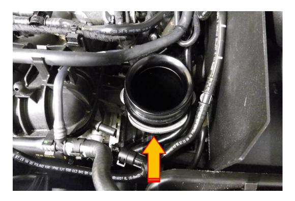
7. Fit the supplied O ring into the machined slot of the smaller two-piece Forge coupler as shown in the picture below.
