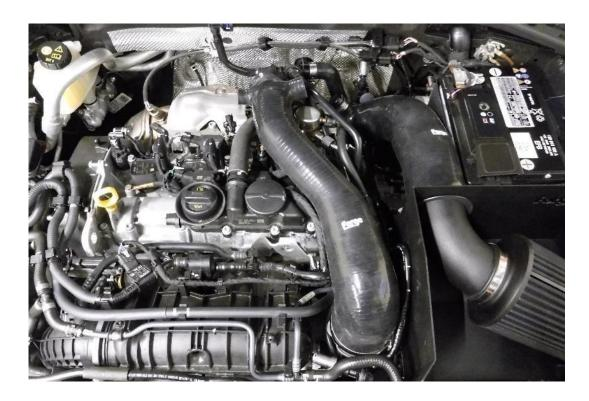
12. If your vehicle is fitted with the extra breather hose you will need to attach the alloy supplied Norma fitting to the 15mm spout, if it does not have this breather then fit the supplied alloy plug. Secure in place with the supplied 12-22mm hose clamp.
