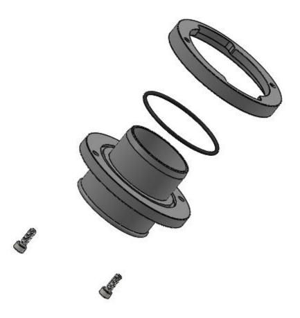
9. Place the two-piece Forge Motorsport billet coupler onto the turbo outlet by locating the two keyway cut outs on the back of the coupler over the tabs on the turbo out-let. Once in place twist either clockwise or anti clockwise as far as possible then tighten the two M4 fasteners with an Allen key.
