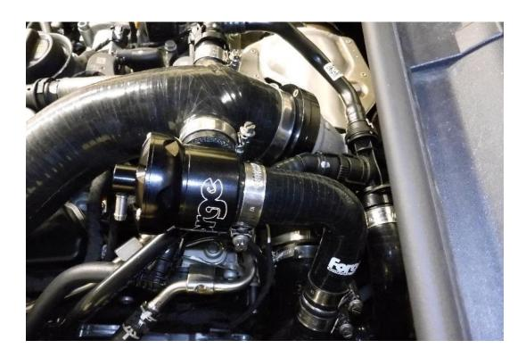
15. Push one end of the supplied silicone vacuum hose onto the Forge vacuum T (from step 10.) and secure it with a cable tie. Run the vacuum hose up to the dump valve and cut to length with scissors or a sharp knife. Use cable ties provided to route it away from any moving parts. The arrows show where to locate the cable ties.
