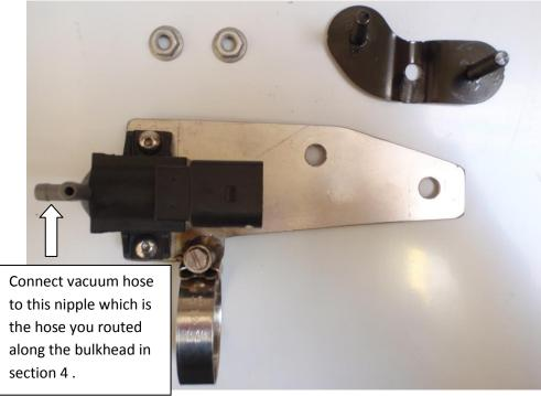
15. Then connect the other vacuum pipe to the solenoid that comes from your boost source, this is the piece of vacuum pipe you fitted to the take off block beneath the battery tray. The image below illustrates the correct way to install all the vacuum pipes.
