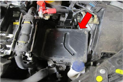
8. Now the battery and plastic tray have been removed, undo the remaining three bolts using a 13mm ratchet.
