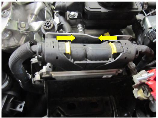
10. There are several plastic clips on the battery tray holding cables etc. These need to be un-clipped to remove the tray completely. Do this by pulling back on the tab to release the 'tooth' as pictured.
