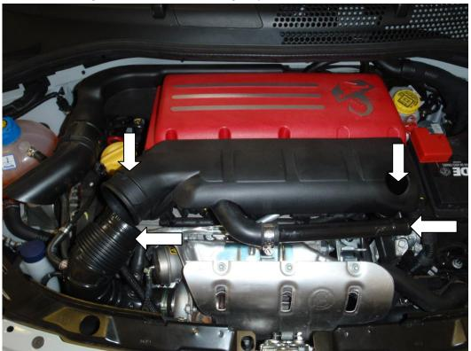
2. Using a T20 screw driver, remove the plastic bracket that retains the 3 hoses next to the oil dipstick, then using a T30 screw driver remove the MAP sensor from the inlet manifold. 1
