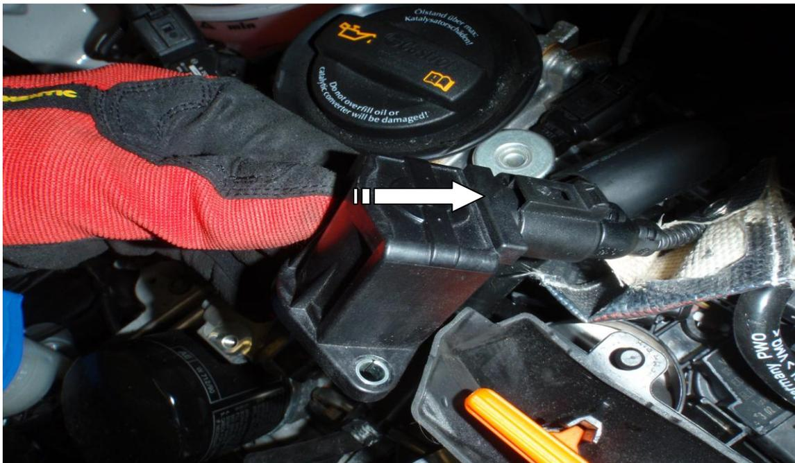
7. Fit the new forge dump valve where the existing standard valve came from using original T30 torx. (If you find this difficult to fit, unscrew the lid on the valve removing it and the spring and then refit once screws have been tightened taking care not to get any dirt in the valve or cross threading the lid when screwing back together).MAKE SURE THE TOP VACUUM PORT IS POINTING AT A 9 o clock POSITION AND THE BOTTOM VACUUM PORT IS POINTING AS SHOWN IN THE PICTURE BELOW
