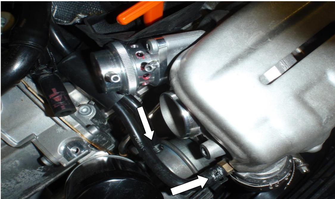
9. Now replace the turbo intake pipe screwing the T30 Torx and pushing the rubber breather pipe back into place, once the rubber breather pipe is on, replace the hose clamp by squeezing the hose clamp together with a pair of pliers back into place.
