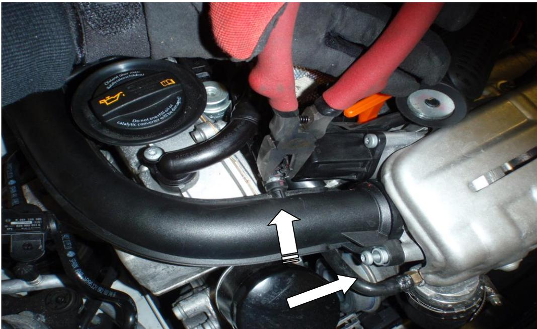
3. Remove the 2 T25 Torx holding the intake pipe bracket on, once the screws have been removed, pull the plastic bracket upwards to remove, this will allow the intake pipe to be removed.
