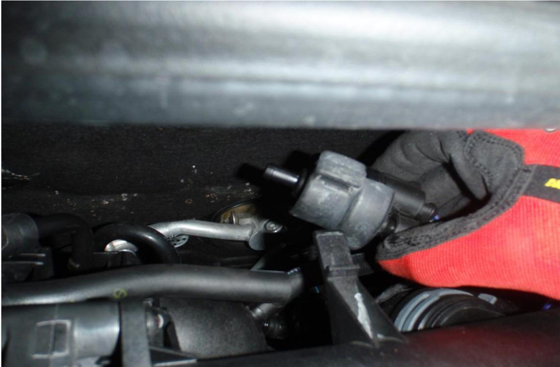
11. Looking directly down from where you have moved the purge valve is a pressure sensor as show in the 2 photos below. Undo both of the T20 Torx holding the sensor to the manifold. Once that is done it will now be easier to remove the plug from the pressure sensor by pressing the tab down and pulling away from you as you did previously on the standard valve.
