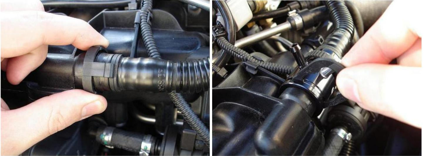
Once the manifold tap is held securely in place with the plastic C-clip, reattach the PCV hose to the barb at the end of the tap. If you are using some sort of PCV “fix” or “bypass”, however, you will need to reconnect whatever components are supplied with that product. The barb on the end of our manifold tap is the same size and shape as the OEM manifold barb, so any hoses or caps that connect to the manifold barb will connect to the barb on our tap as well.
