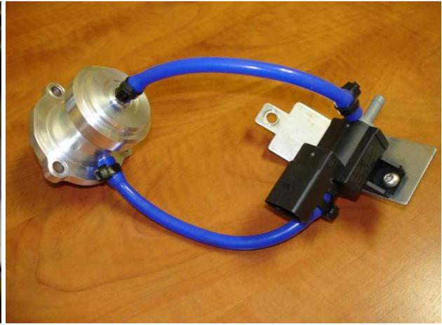
With the new Forge valve loosely mounted to the turbo, and a location selected for the solenoid and it loosely mounted as well, measure to find appropriate lengths for the vacuum hose connections between the valve and the solenoid.
