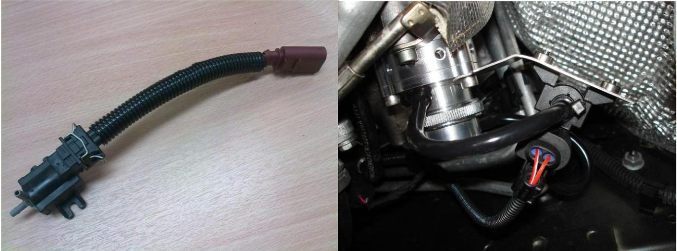
With the valve securely mounted to the turbo and the solenoid bracket also secured at your desired location within the engine bay, you can reconnect the OEM wiring harness plug to the connection on the end of the Forge wiring harness.
