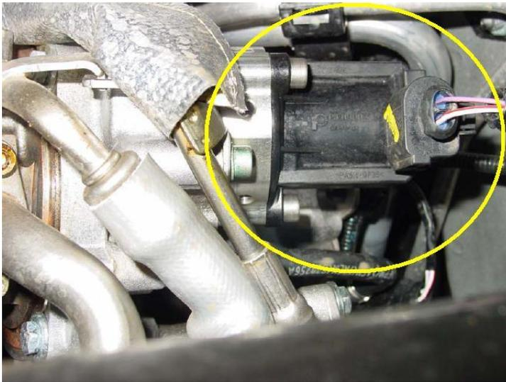
Once located, disconnect the electrical connector/plug for the valve and you can now use your 5mm Allen wrench or socket to remove the three 5mm Allen bolts which secure the valve to the turbo. You must be sure to save the OEM valve bolts as they will be reused later.
