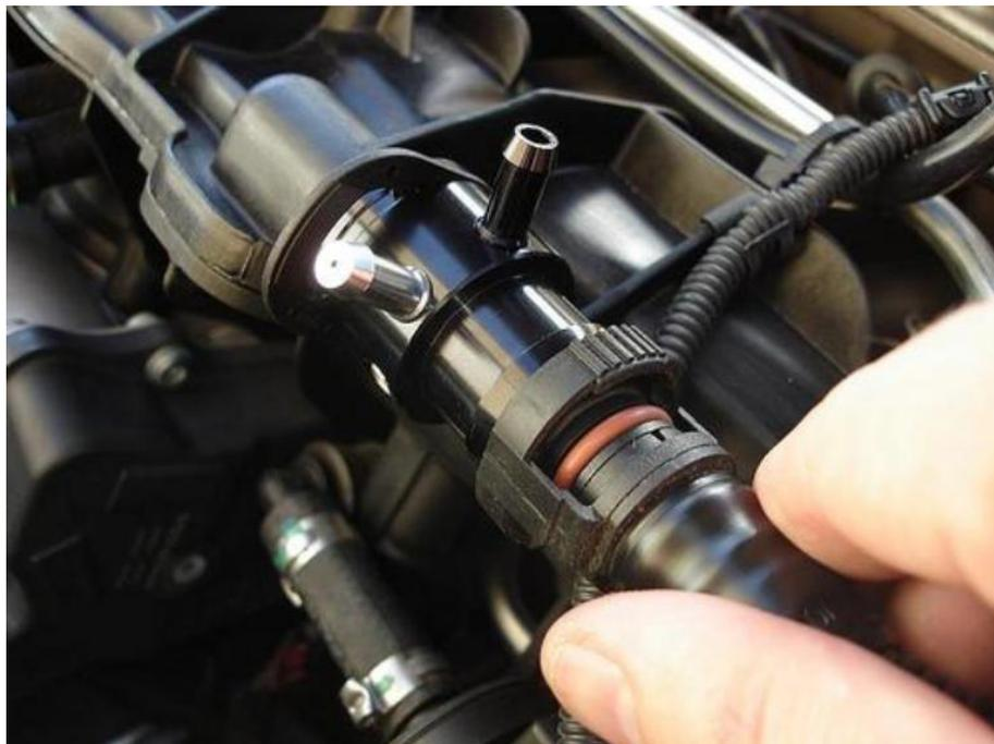
From the appropriate nipple on the manifold tap (largest port), run a length of vacuum tubing along the top of the motor, around the passenger side, following the fuel rail and fuel lines, down to the remaining linear port on the solenoid you mounted previously. (See plumbing diagram) Secure both ends of this line using two of the included zip ties. If any spare zip ties are available, use them to secure this vacuum line to the fuel rail and/or fuel lines.
