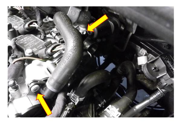
**10**. Fit the FMTIA3 hose to the turbo, use the supplied 40-60mm hose clamp to secure it in place. Note that the hose clamp and silicone hose should be as close to the face of the turbo as possible.
