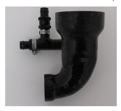
8. For cars with the additional breather, you **MUST ENSURE** that the part is orientated correctly. There is a flat on the part as shown below. Orientate the flat so that it is in line with the vertical hole for the one-way valve. You will be able to see the hole in the breather adapter through the one-way valve hole.
