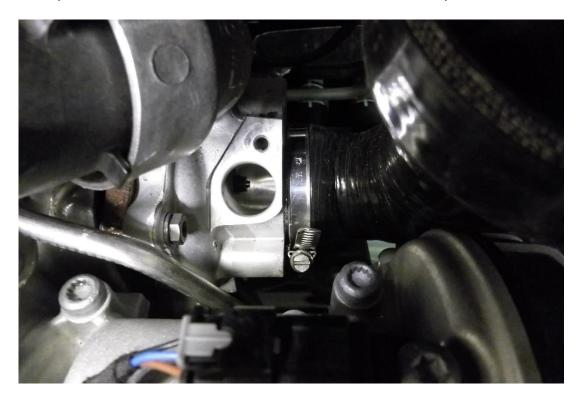
11. Re connect the breather pipes to the machined fittings on the FMTIA3 hose. And re fit the oil breather hose.
