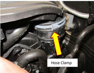
3. Pull the airbox Sharpley in an upwards motion to remove it from situ.
