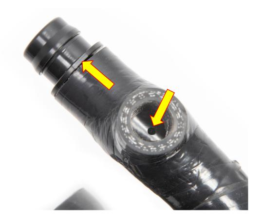
9. Using a T30 Torx drive remove the fasteners that hold the oil breather hose in situ. The breather hose can now be removed.
