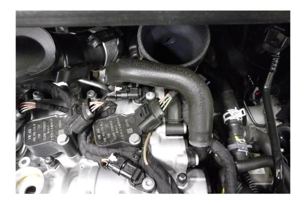
12. Attach the air box to the FMTIA3 Hose using the supplied 70-90mm hose clamp then push the air box back into position. We would advise lubricating the rubber mounting points of the airbox as this will help with re installation. Re fit the breather hose and the T25 fastener removed from step 1&2.
