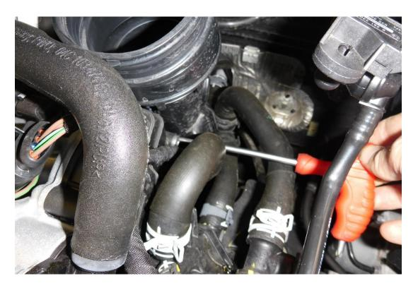
5. Disconnect the breather pipes if your vehicle is equipped with this system. Simply push in both side tabs and pull the pipe off the fitting. Remove the loom going to the turbo actuator, press the tab in on the pug and pull away.
